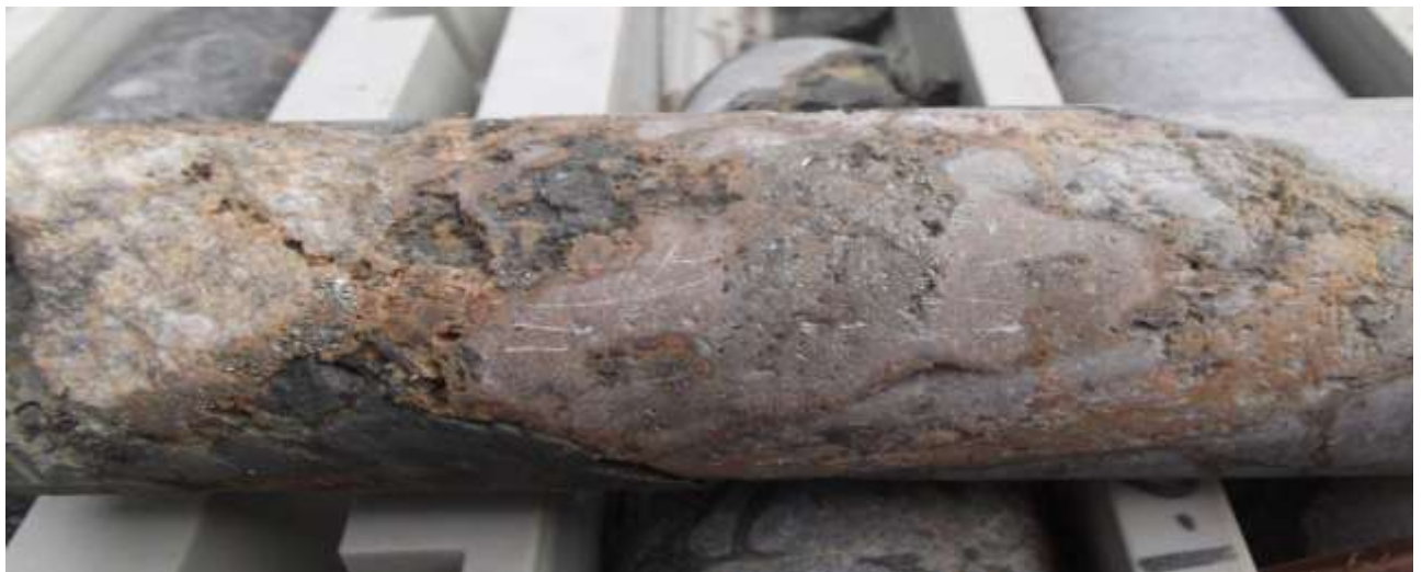
Photo 4: Quartz- pyrite-kfeldspar/siderite? breccia band from 360.90-361.10m. Notice the pyrite bleb in the centre of image and orange yellow k-feldspar (?) and or siderite?
