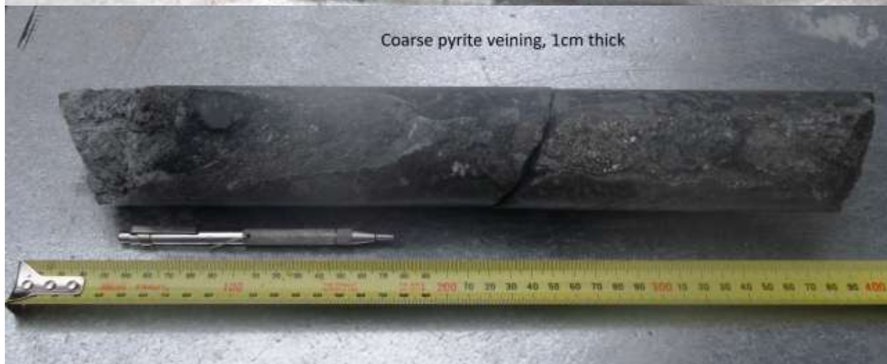
Photo 1a and b: Vein extends up to 30cm and infill with semi-massive coarse pyrite (>10%) grains and quartz, k-feldspar and carbonate, range between 576.70 – 577.60m.
