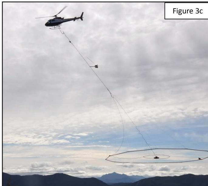
*The system was designed to be field configurable to best suit a large variety of different geophysical requirements from deep penetration to optimizing the discrimination within a narrow range of resistivity values.*
